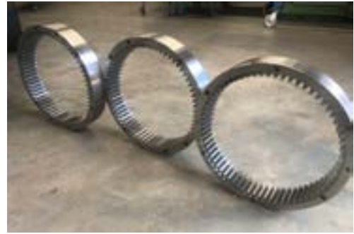
600mm diameter internal clutch rings
