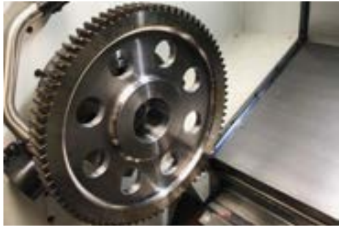
Large gear final machining on lathe
