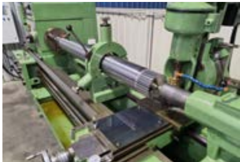
2500mm spline shaft cutting
