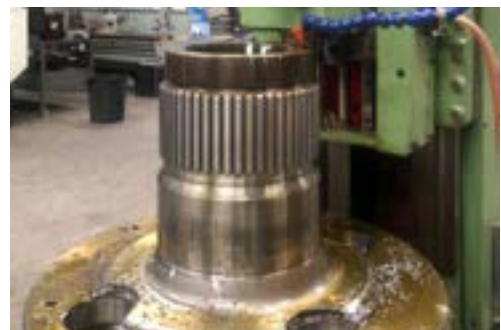
Planet carrier spline cutting
