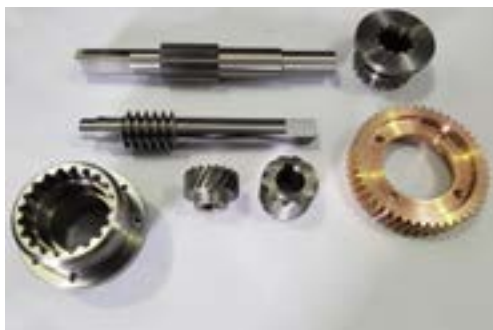
Gearbox components for a submarine
