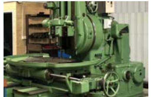
Our MAAG SH150/180 capable of cutting gears to 1.8m diameter
