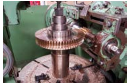
EN12 Lorenz Hobber cutting a worm gear
