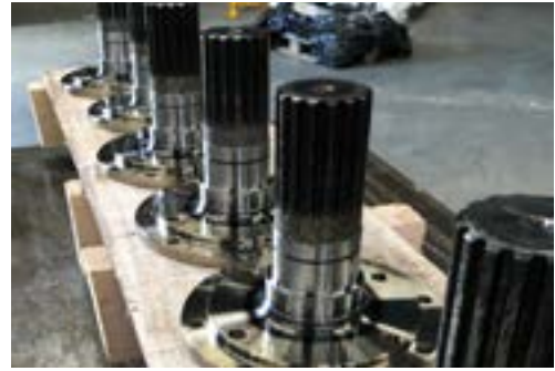
Pump box input shafts
