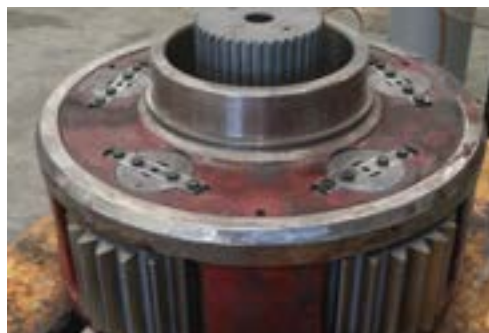
Planetary reducer gearbox final stage
