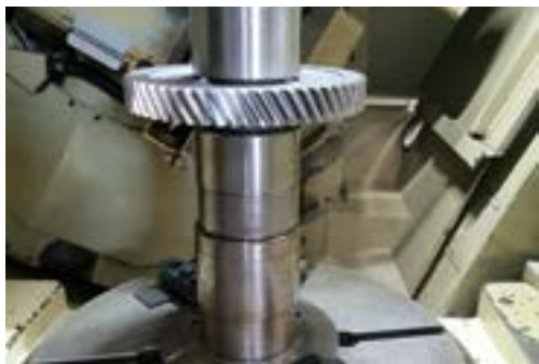
Helical gear grinding
